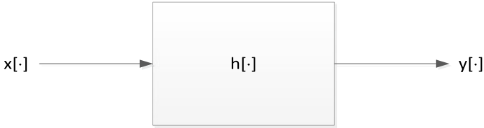
Fig. 1.12 Digital filter block diagram
